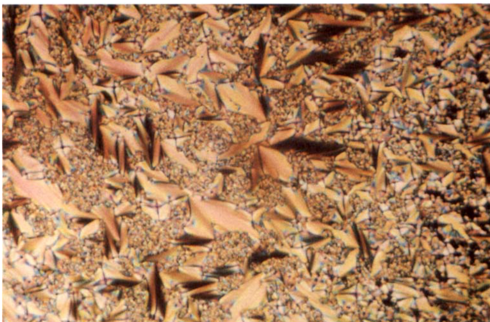
Figure 3. Photomicrograph of the smectic A phase of polyacrylate H6 (crossed polarizers; 71°C).
